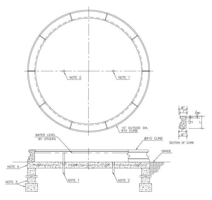
POOL CURBING SETTING and RECOMMENDED WATERPROOF MATERIALS In order to properly set and waterproof the seams between the curbing sections and the concrete pad, we recommend that the following instructions be followed: Prepare wood wedges 4" long tapering 0" - 1".
